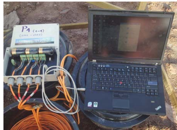
Instrument installation and dam performance monitoring at Phu Kham mine tailings dam All capable of being raised as the elevation of the dam is increased over time - Lao PDR
