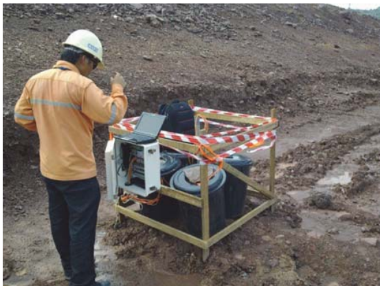
Instrument installation and dam performance monitoring at Phu Kham mine tailings dam All capable of being raised as the elevation of the dam is increased over time - Lao PDR
