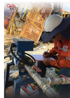
Computer controlled insitu permeability testing and grouting instrumentation for mining project in the Lao PDR
