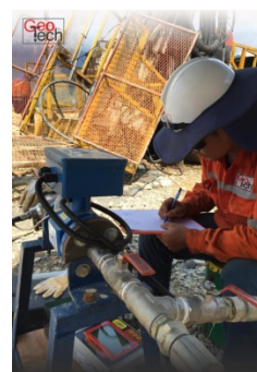
Computer controlled insitu permeability testing and grouting instrumentation for hydropower project in Lao PDR
